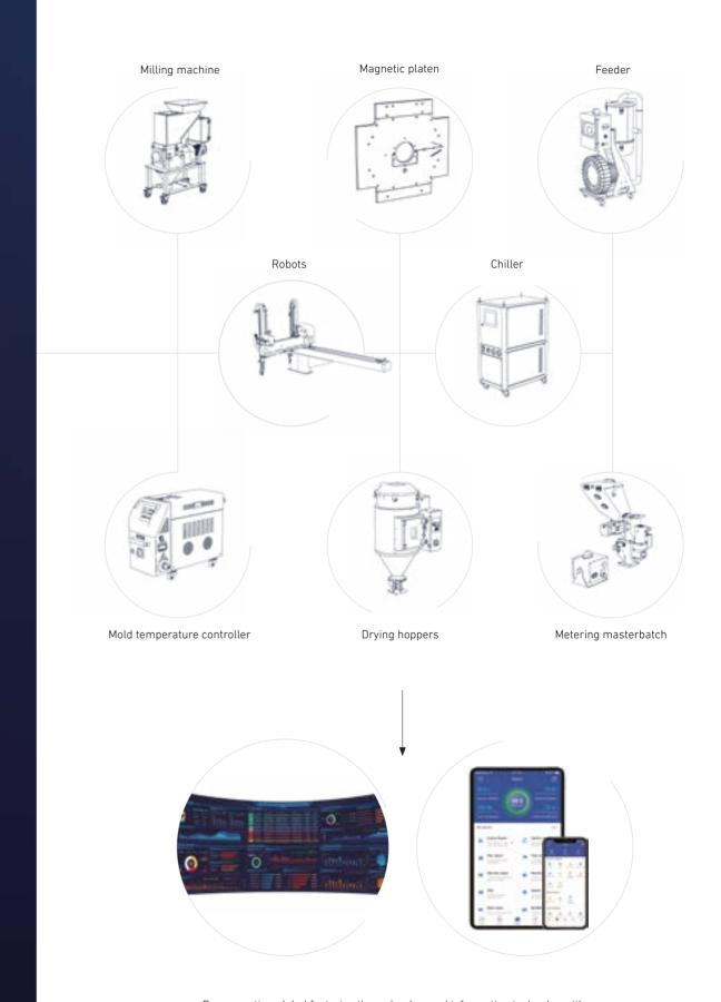
By connecting global factories through advanced information technology, it's possible to monitor the operational status of all factories and each injection molding machine worldwide from a central monitoring hub.
