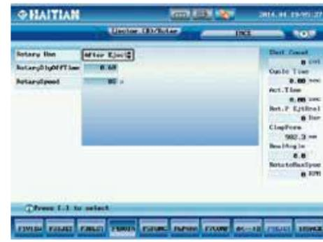
The control system of the servo hydraulic turntable is equipped with a rotating encoder, which provides immediate feedback on the turntable location. By changing the degree of opening of the turntable's proportional direction valve as well as the system's pressure and flow, the closed loop control is established.
