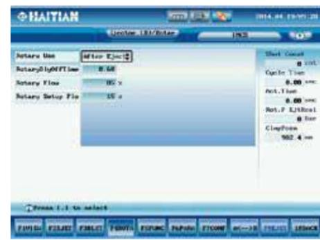
The servo motor turntable system is equipped with an electric servo motor and inverter, to feedback on the turntable position, by changing the speed and torsion of the electric servo motor, the closed loop control is established. The servo motor electrical turntables has got the advantage of speed, stability and precision.
