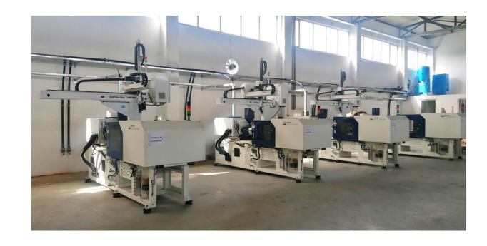
Installed the largest electric injection molding machine in Europe – ZERES III with 1380 tons of closing force
